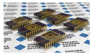
The world's first diamond semiconductor amplifier circuit has successfully demonstrated reliable operation under high temperature, specifically for a week at 300°C. This achievement marks a significant milestone towards the practical application of diamond semiconductor devices.
