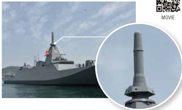
Integrated multiple antennae, covered with low RCS Radome. Advanced stealth technology required for the mast of brand-new frigates is realized by gathering Japanese technologies. Introducing UNICORN, the embodiment of excellent technologies.
